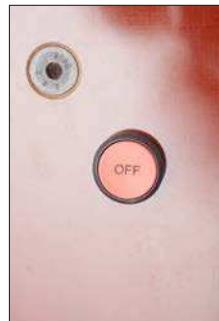
Fig.18 – Emergency STOP button at the front of the coil
