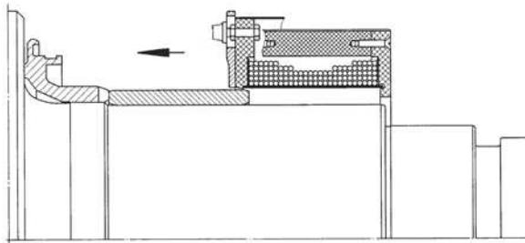
Fig.10 – The heater is being positioned over the ring
