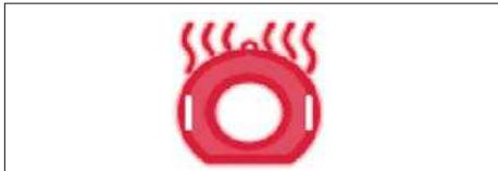
Fig.17 – Too hot coil warning symbol
